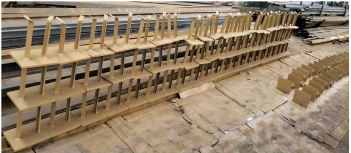
Embedded Part for Crane Beam
