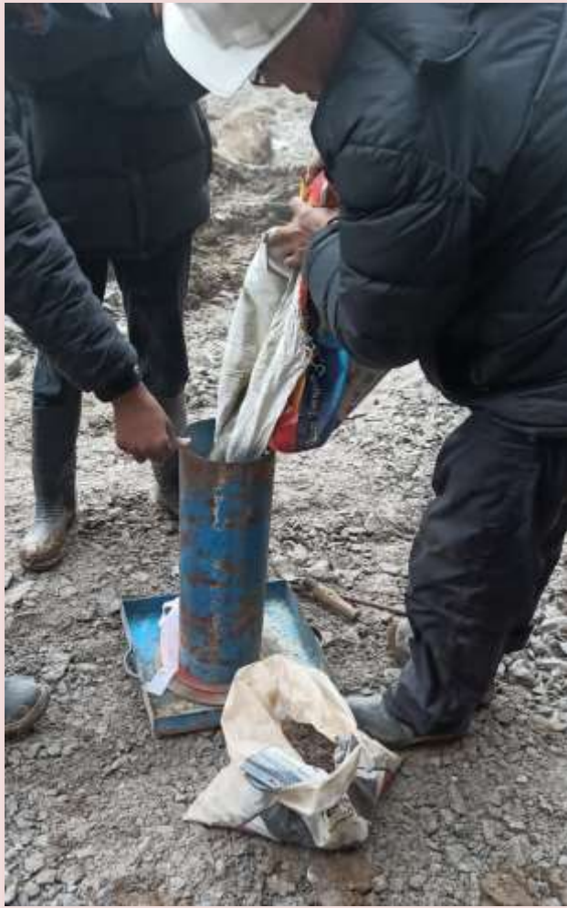
Field Density Test for Foundation of Transmission line(Left) Placement of rebar in foundation(right)
